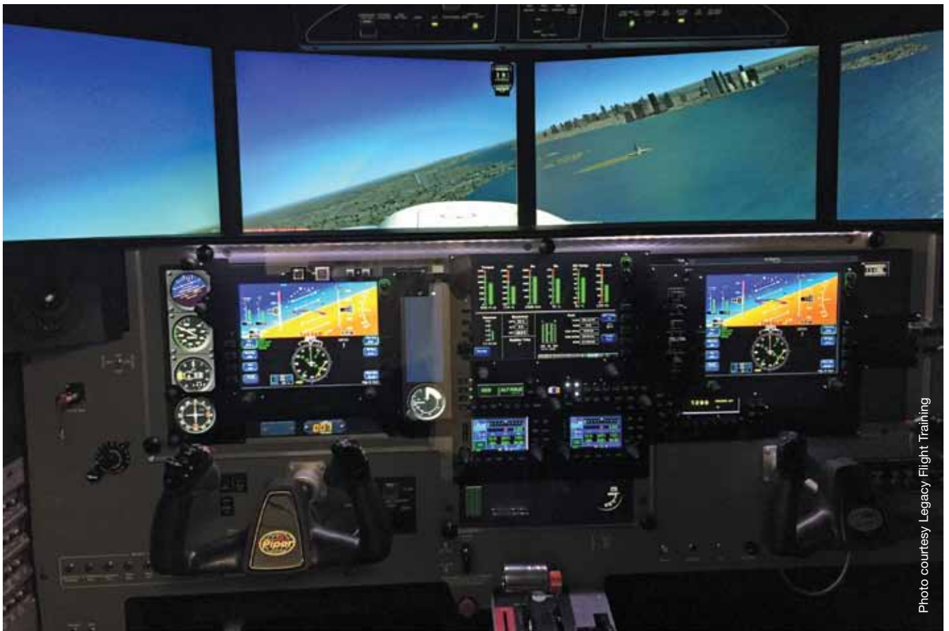
Legacy Flight Training offers pilots a Meridian simulator with Avidyne avionics.
