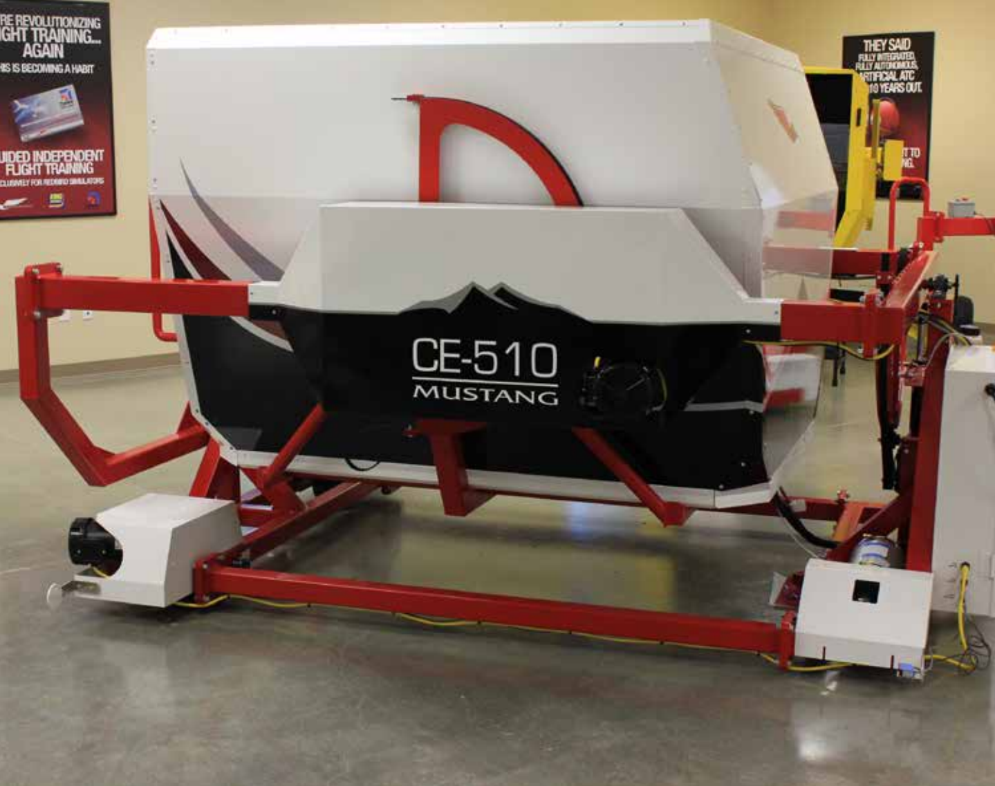
ABOVE: When Redbird started making full-motion sims, it was for simple airplanes. Today, much of the business the company does is making full-motion simulators for turbine aircraft. Two of its most popular models are the Cessna Mustang and the CitationJet.
