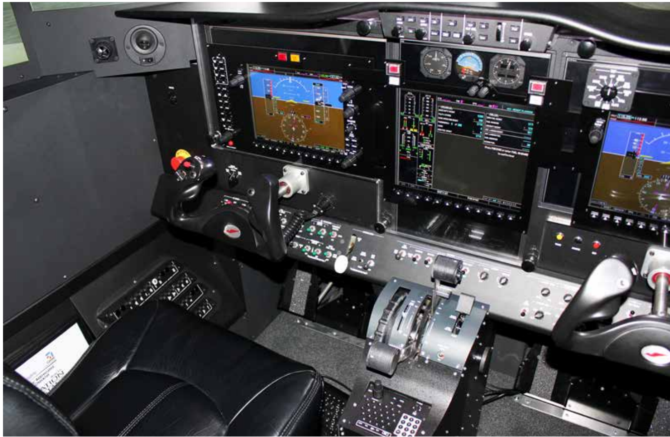
ABOVE: The cockpit of the Cessna Citation Mustang is all business, with the look and feel of the real McCoy. Companies like Angel City Flyers use the Mustang flight training device to simulate failures and in the process greatly reduce the amount of time, and dollars, prospective PICs spend in the actual airplane.
